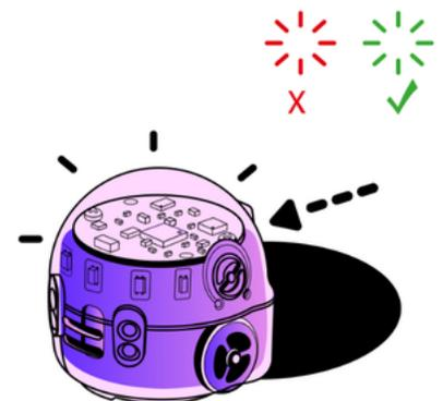
Calibrate: adjust or set up the Ozobot so it can work properly by recognizing its environment—like making sure it can see and follow lines or colors correctly
